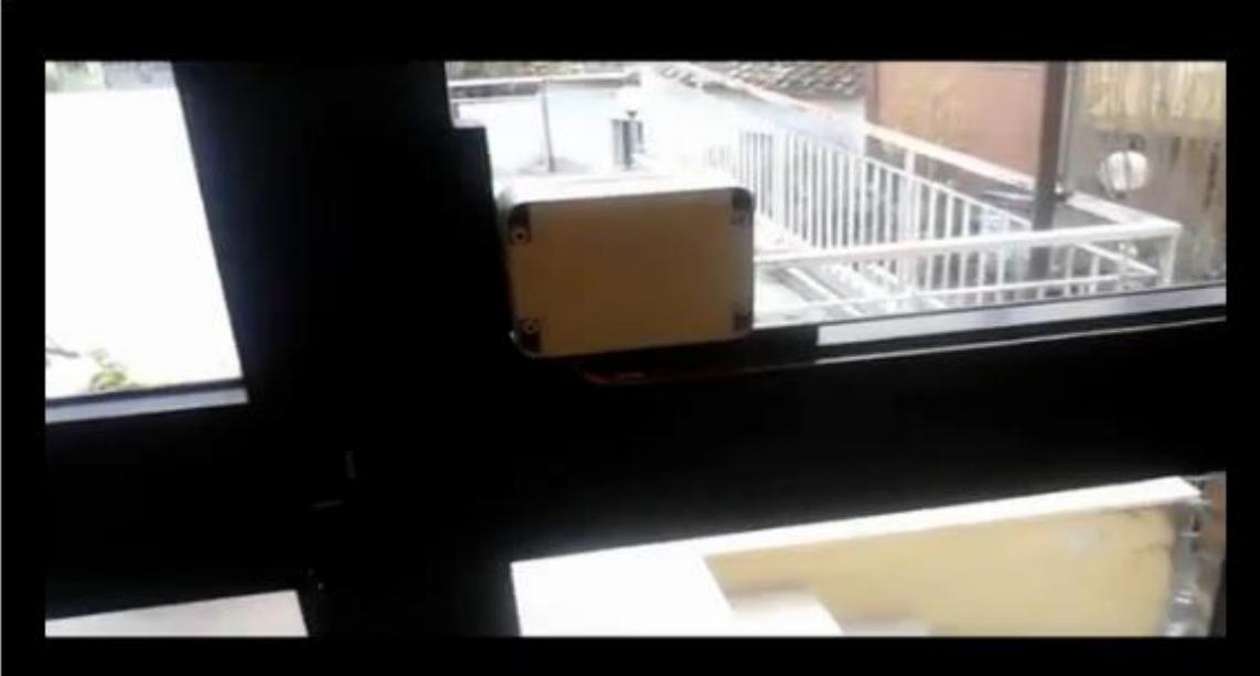
The bracket is more long than the box so, once you have screwed the box to it, you can further screw the bracket to the door.
